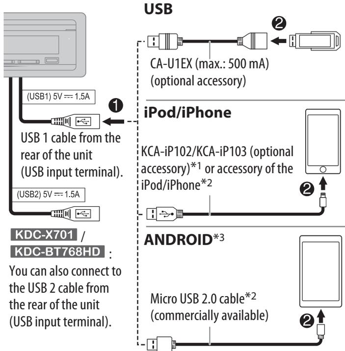
\*1 KCA-iP102 : 30-pin type, KCA-iP103 : Lightning type
